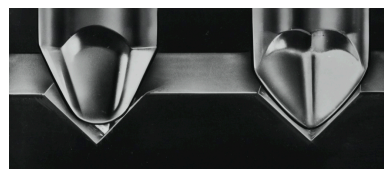
Figure 3.18: An example of an elliptical stylus on the left vs. a line contact Pramanik grind on the right. Notice the difference in the area of contact between the styli and the groove walls.
