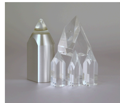
Figure 3.19: Scale models (on two different scales) of different styli. The example on the left is bonded, the other four are nude.
