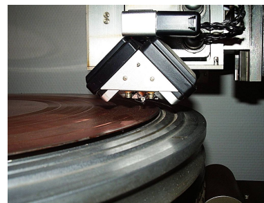
Figure 3.11: A Neumann-Teldec cutting head creating the groove in the master disc. The cutting stylus shown in Figure 3.10 can be seen just under the circular support under the head. (Wikimedia Commons)
